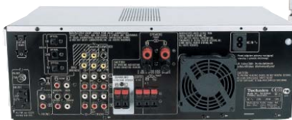
Amplituner Technics SA-DX940. Zawiera dekodery Dolby Digital i DTS. Moc 5x50W cena 1700 PLN
